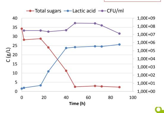
→ SHF at low total sugar and using hydrolysates in batch yields 70-80% D-lactic acid at 45 °C
