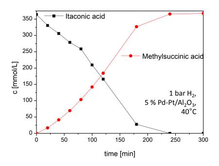
Standard reaction conditions: 400 mL 5 % IA solution,  $\rm H_2$ -pressure, 1 g 1-5 % metal/ $\rm Al_2O_3$ , 40-80 °C
