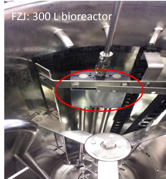
**Monitoring gradients by multi-position sensor (pH, pO<sub>2</sub>) in 100 and 300 L bioreactors at TU Berlin and FZ-Jülich**
